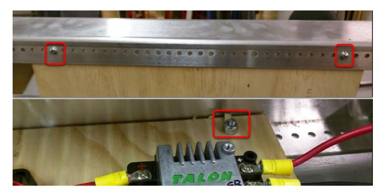
Requires: (4) 10-32 x 1" pan philips head machine screw, (4) 10-32 nylock nuts (there should be extra in the drive base kit), philips head screw driver, wrench
