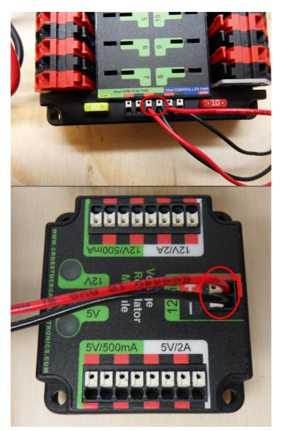
Requires: Wire stripper, small flat screwdriver (optional), 18AWG red and black wire
