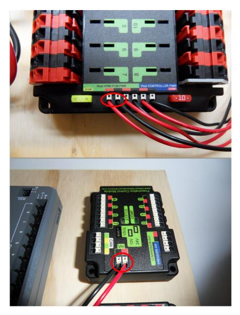
Requires: Wire stripper, small flat screwdriver (optional), 18AWG red and black wire
