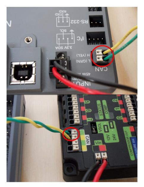
Requires: Wire stripper, small flat screwdriver (optional), yellow/green twisted CAN cable
