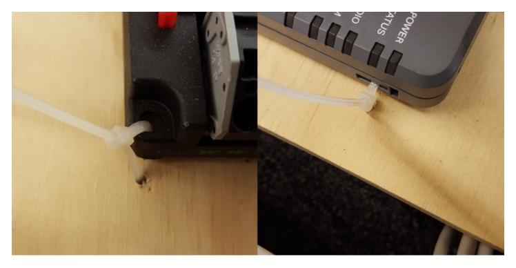
Using the Dual Lock or hardware, fasten all components to the board. Note that in many FRC games robot-to-robot contact may be substantial and Dual Lock alone is unlikely to stand up as a fastener for many electronic components. Teams may wish to use nut and bolt fasteners or (as shown in the image above) cable ties, with or without Dual Lock to secure devices to the board.
