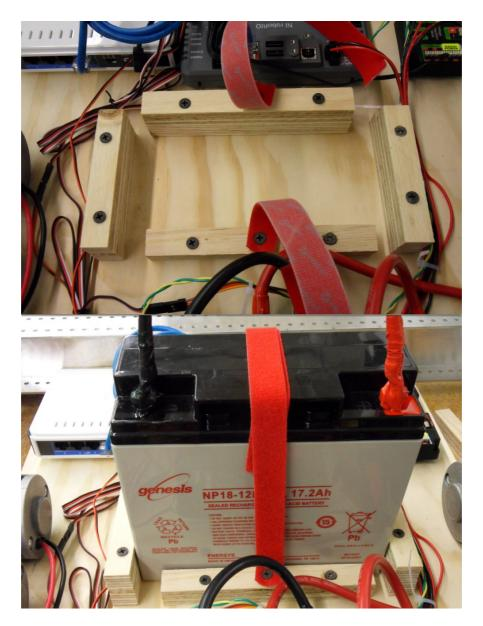
Requires: Plywood Scraps, plywood cutting tool (e.g. saw), 10x 2" wood screws, drill, 1/8" drill but, Philips head driver bit or philips head screwdriver, velcro wrap
