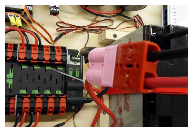
Connect the battery to the robot side of the Andersen connector. Power on the robot by moving the lever on the top of the 120A main breaker into the ridge on the top of the housing.
