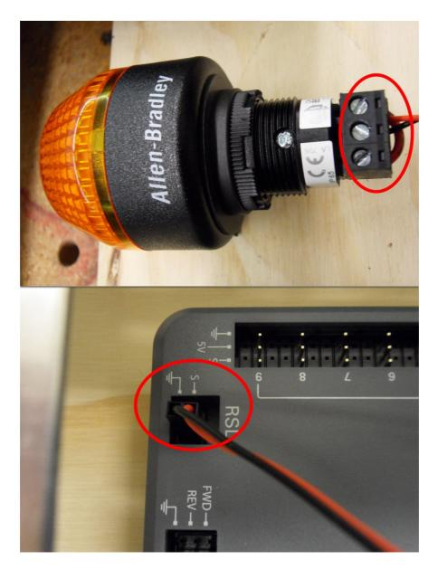
Requires: Wire stripper, 2 pin cable, Robot Signal Light, 18AWG red wire, very small flat screwdriver
