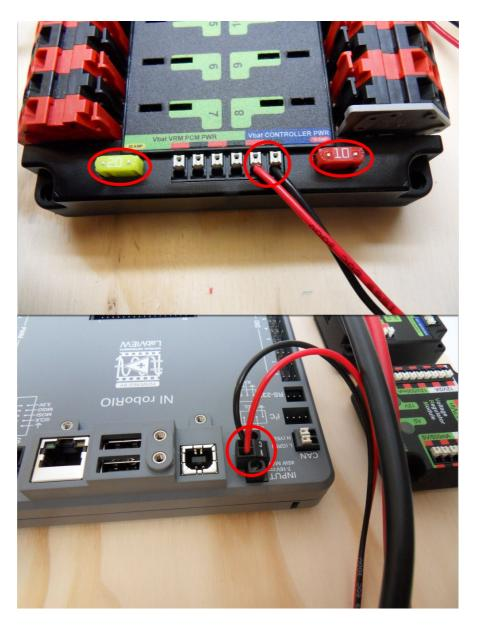
Requires: 10A/20A mini fuses, Wire stripper, very small flat screwdriver, 18AWG Red and Black
